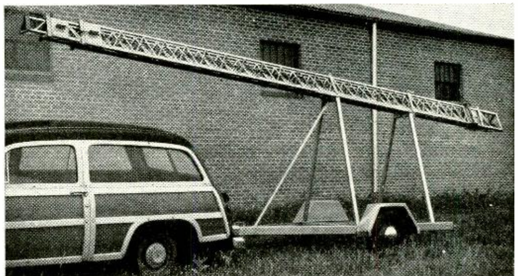
Fig. 1 (opposite)—Collapsible 80-foot mast finds best antenna height at customer's site, doubles as derrick for raising permanent tower. Fig. 2 (right)—The aluminum test tower in transport position—ready to roll to another customer-home demonstration.
