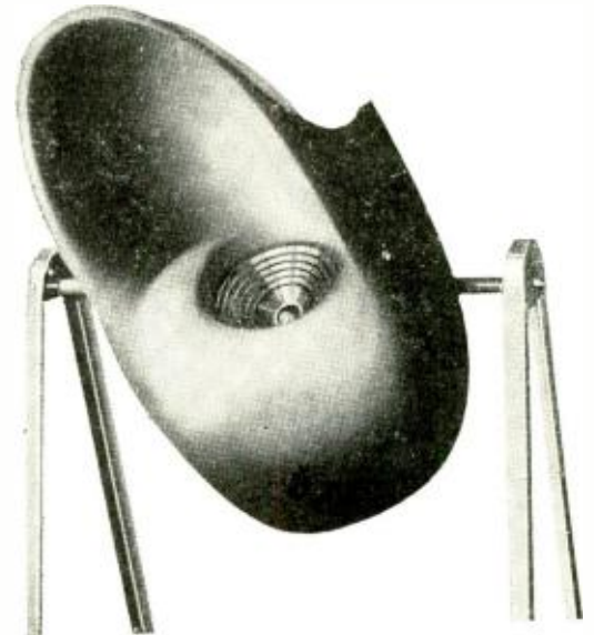
Large sound mixer baffle (Pathe type) used in French film-theatre sound systems.
